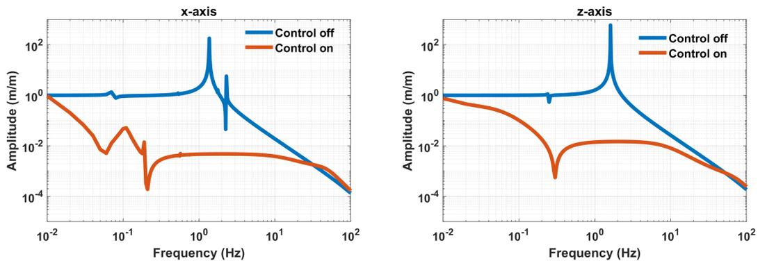
Figure 2.12: Transmissibilities from Ground to AP.
