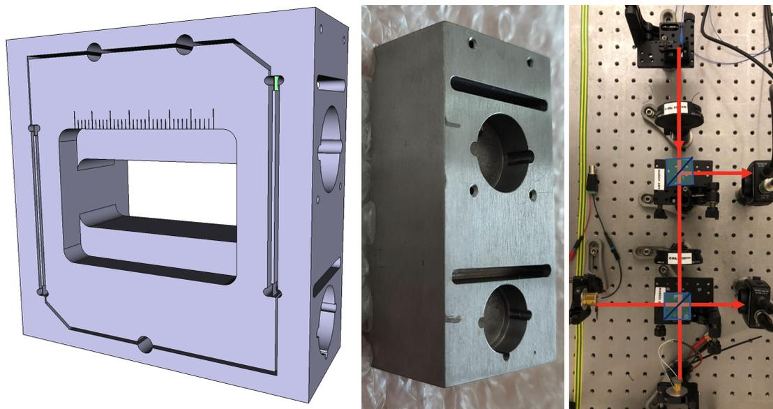
Figure 2.52: Current status of CSIS: (left) CAD render of the monolithic sensor mechanics with one of the eight  $100 \mu\text{m}$  thick flexures highlighted in green, (middle) a photograph of a niobium test block with the upper readout hole and lower actuator hole and (right) a top view of the interferometric readout.
