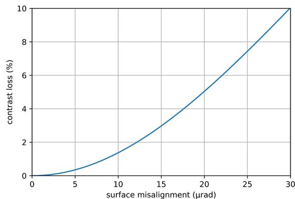
Figure 3.19: Loss of interference contrast for misalignment of the two surfaces of the silicon test mass. To keep loss to less than 10%, any wedge of the test mass must remain less than around  $30 \mu\text{rad}$  (ca.  $0.10$  arcmin).
