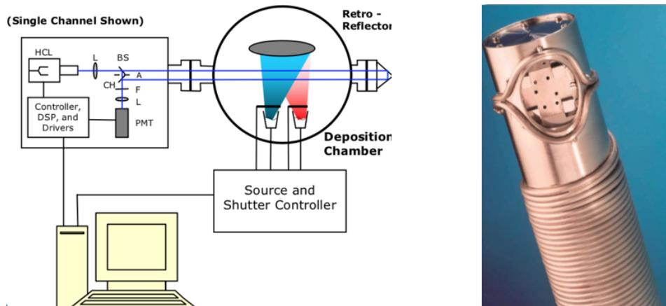
Figure 3.10: An implementation of AAS (left) and a picture of a cross-beam ion source as part of a QMS system (right).
