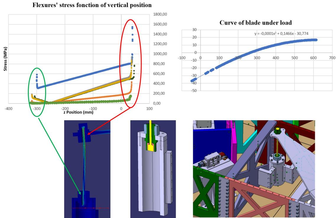
Figure 2.28: Finite Element Analysis of the Flexure.
