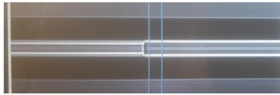
Figure 3.3: Ho:YAG crystals to be used for the ring oscillator
