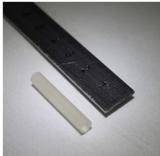
Figure 3.2: Ho:YAG crystals to be used for the ring oscillator
