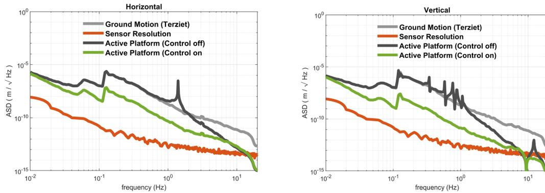
Figure 2.3: Active Platform Motion of E-TEST Isolation System.
