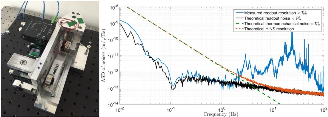
Figure 2.31: Horizontal Interferometric Inertial Sensor (HINS) [17]. Sensor (left) and performance (right). It is characterised by a resonance frequency of 0.11 Hz and a Q-factor of 20. It is achieving sub-pm resolution above 0.01 Hz.
