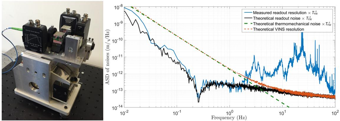
Figure 2.32: Vertical Interferometric Inertial Sensor (VINS) [17]. Sensor (left) and performance (right). It is characterised by a resonance frequency of 0.25 Hz and a Q-factor of 30. It is achieving sub-pm resolution above 0.01 Hz.
