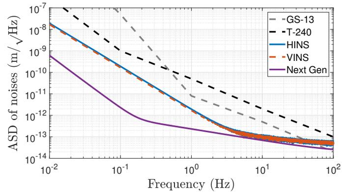
Figure 2.33: Prototype of the next-generation VINS sensor. Using new, high-performances, photodiodes and considering reduced thermal-noise in the UHV environment, the performances can be improved by 1 order of magnitude below 1 Hz, and by a factor of 2 above 1 Hz.
